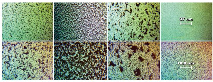
Microscopic images of 8% Unipure Red LC381 AS-EM in Octyldodecanol, TGI, Castor Oil and CE-2000 (from left to right) Magnification: top, 100X; bottom, 2500X
